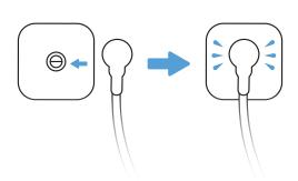
3 Attach wire to pads by snapping leads onto pad terminal.
