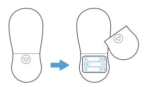
Remove the battery cover and insert three AAA batteries into the battery holder, observing the polarity.
