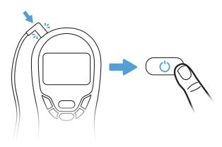
**5** Connect wire to device and power on.
